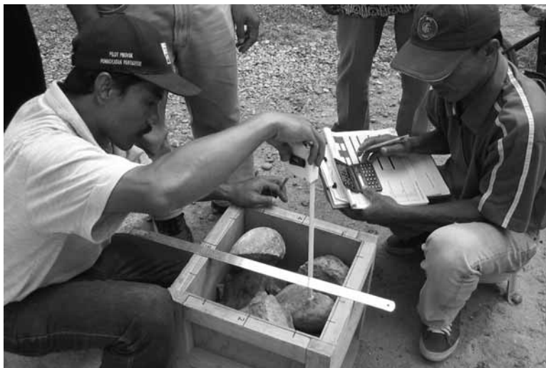
To test for corruption, auditors measure the materials used to resurface a road in Java, Indonesia.
